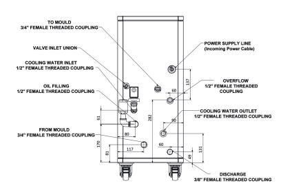
Thermotech Power oil mold temperature controllers with indirect cooling are used in various industries, particularly in injection molding, to maintain the optimal temperature of molds during production processes.
