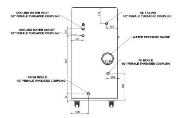
Thermotech Power Plus mold oil temperature controllers are specialized devices used in industrial processes such as injection molding, die casting, and other applications where precise temperature control of molds is required. These controllers use oil as the heating medium, which can achieve and maintain higher temperatures compared to water-based systems.
