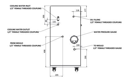
Thermotek EX mold oil temperature controller designed to operate at temperatures up to 300°C is specifically engineered for high-temperature applications in industries such as injection molding, die casting, and other processes requiring precise thermal management.
